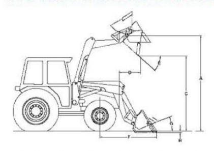
Bucket Capacity =0.5cbm Lift Capacity =1000kg Time to raise boom =10sec
