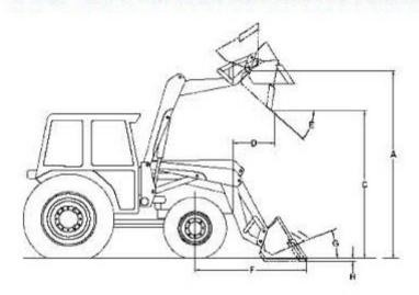
Bucket Capacity =0.23cbm Lift Capacity =300kg Time to raise boom =8sec
