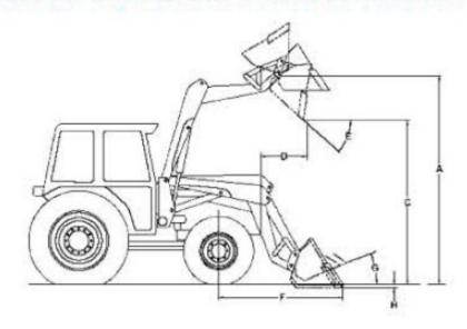
Bucket Capacity =0.4cbm Lift Capacity =800kg Time to raise boom =10sec
